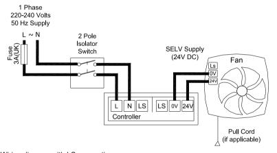
Fig 10. Wiring diagram with LS connection.
